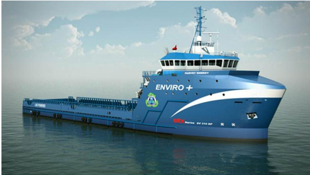
LNG-powered Offshore Supply Vessels like this one will support Shell's operations in the Gulf of Mexico. Image courtesy of Harvey Gulf International Marine.
